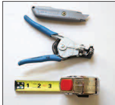
Tape measure, utility knife and wire stripper
