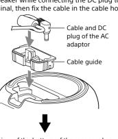
Top view of the bottom of the rear speaker
