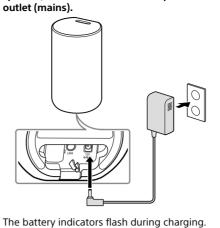
The battery indicators turn off after completion of charging
