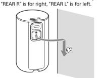
5 When mounting the rear speaker on the wall with the AC adaptor connected, fix the cable of the AC adaptor in the cable holder on the
