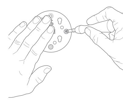
Attach the base of Spotlight Cam to the mounting bracket
